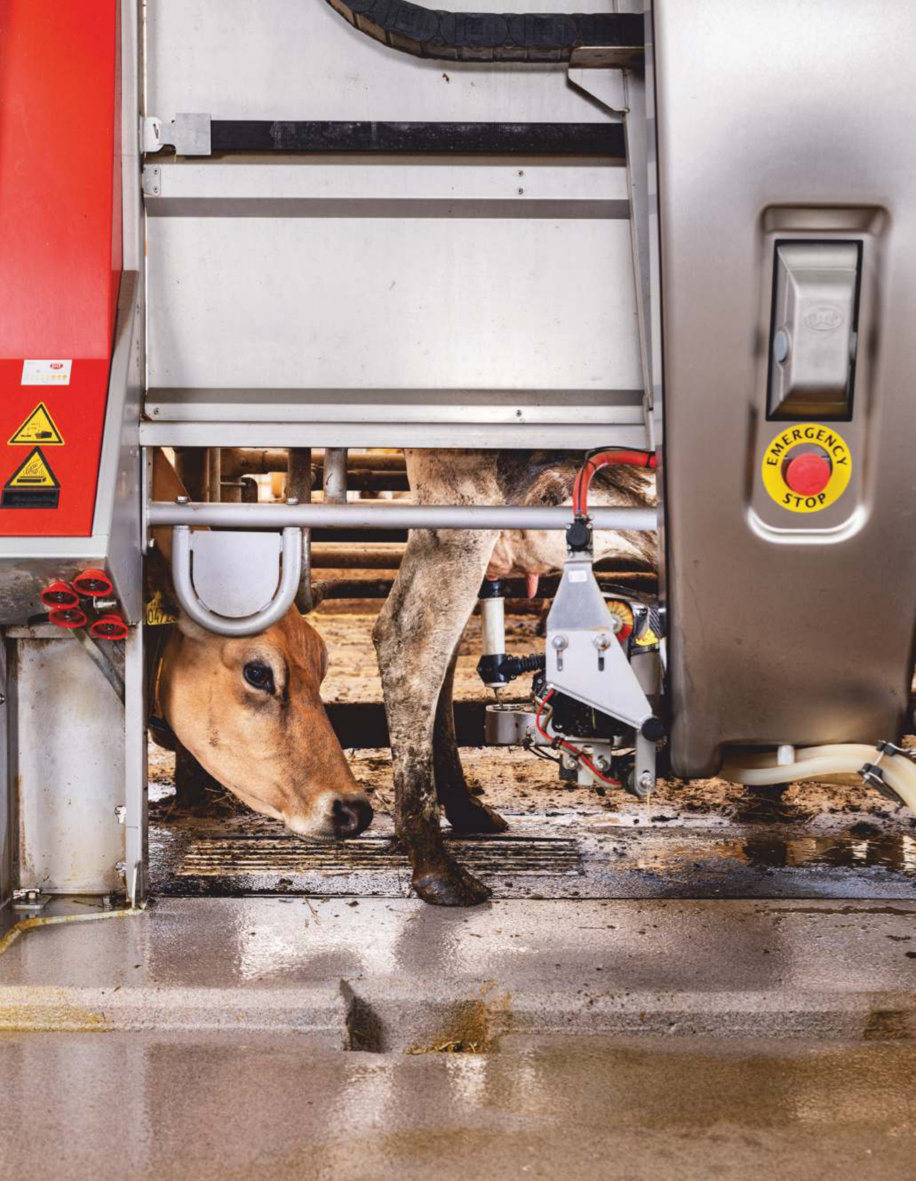
A4 robot. When the animal walks up, the robot scans her collar and gives her a treat if she's right about needing to be milked (if she's not, she gets no treat and walks on). The machine does the milking automatically. Farmers monitor production and give the robot instructions via a touchpad.
